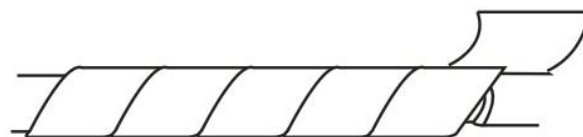
Figure 3.2.2 Third step during wiring – wrapping of insulation layers
